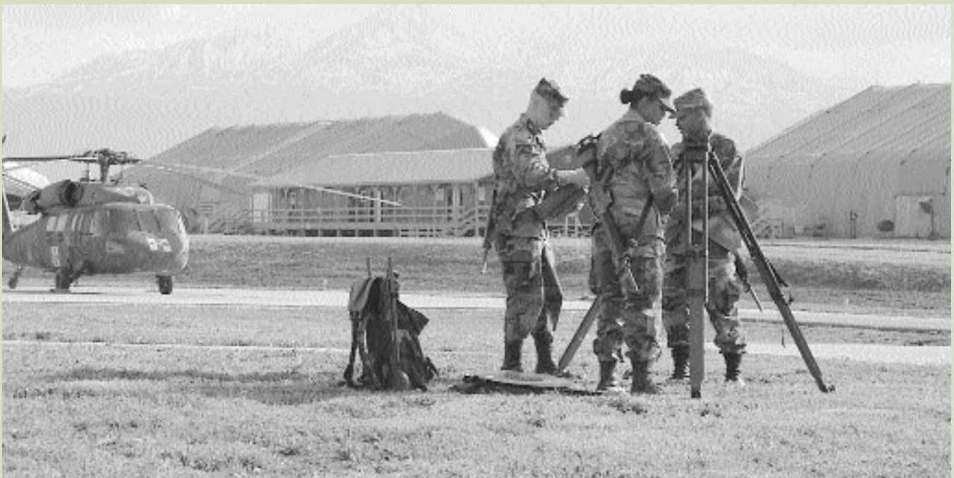
Soldiers of the 320th Engineer Company set up a positioning receiver to survey the airfield, Camp Bondsteel, Kosovo. The low building in the left, center, is a SEA hut.
