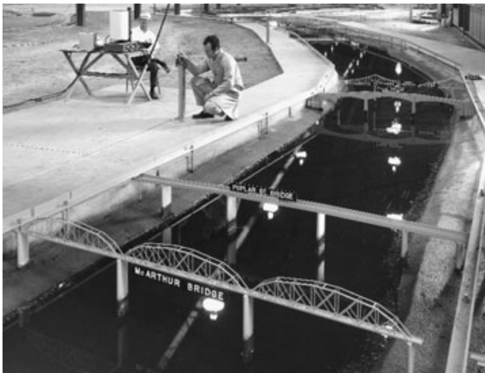
Before computer modeling, the Waterways Experiment Station in Vicksburg, Miss., used physical models to study waterways problems. This model of the Mississippi River at St. Louis, Mo., tested various measures to reduce siltation in the harbor.
