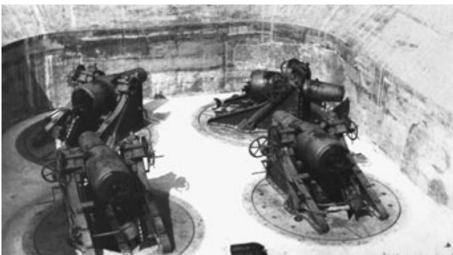
(top) Ten-inch disappearing gun of the Endicott system in the loading position at Sandy Hook, N.J.
