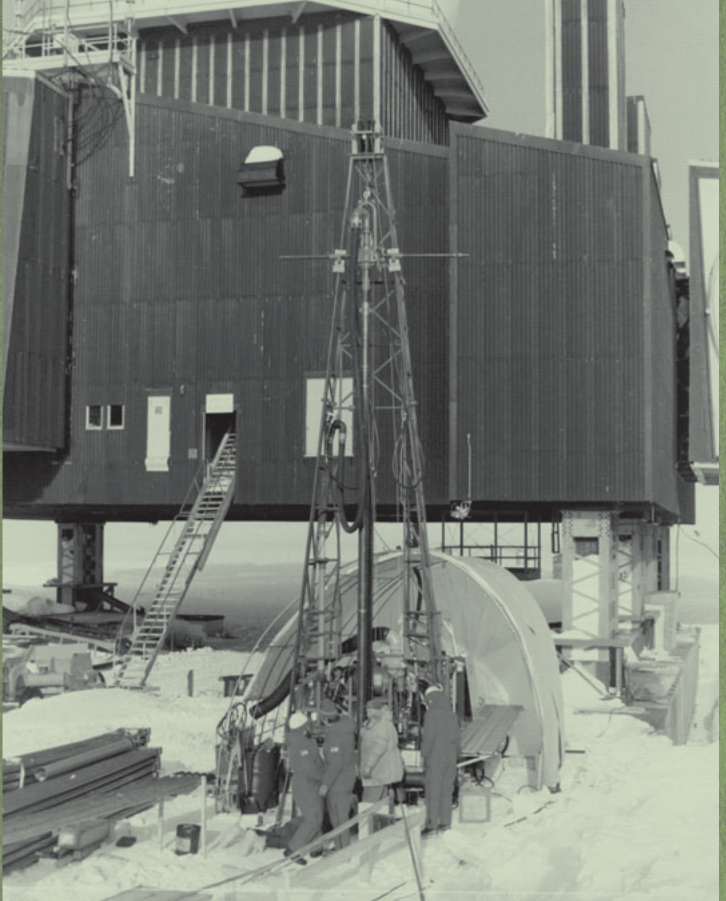
Greenland Ice Sheet Project (GISP), Deep Drilling Operation by the Corps' Cold Regions Research and Engineering Laboratory, 1975. Cold War strategic interest in cold regions prompted extensive research.
